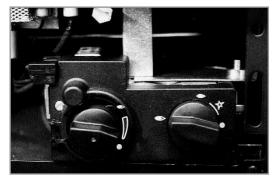
Continue pressing down the knob while turning further to the left to activate the piezo spark, continue to hold the knob down for a further 10 seconds after the pilot has been lit. If the pilot does not light repeat the previous steps.
