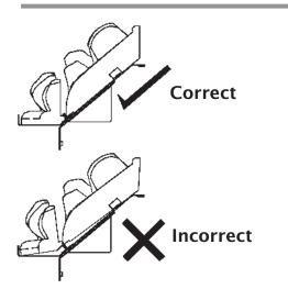
2. Next, remove the front coal strip from its protective packaging and position as shown. The rear edge of the front coal strip should fit in front of the burner rail. Again, do not to place on top of the burner rails. When the front coal is in position bend up the three metal tags at the front of the tray to retain (inset).
